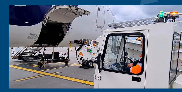
The Assisted Docking System is an aircraft damage prevention system designed to enhance docking safety and efficiency. The system assists the driver in the safe aircraft approach and docking of the Rollertrack Conveyor onto the aircraft door sill. It is based on advanced LiDAR technology and complies with IATA AHM 913 standards.
